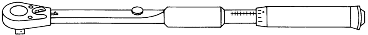
Figure 9. Type III, class 2 torque wrench, - rigid case, micrometer-style torque presetting, audible signal ratchet reversible head.
